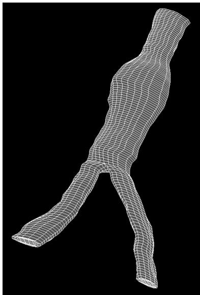
**Figure 11** - Blood vessel bifurcation finite element model
